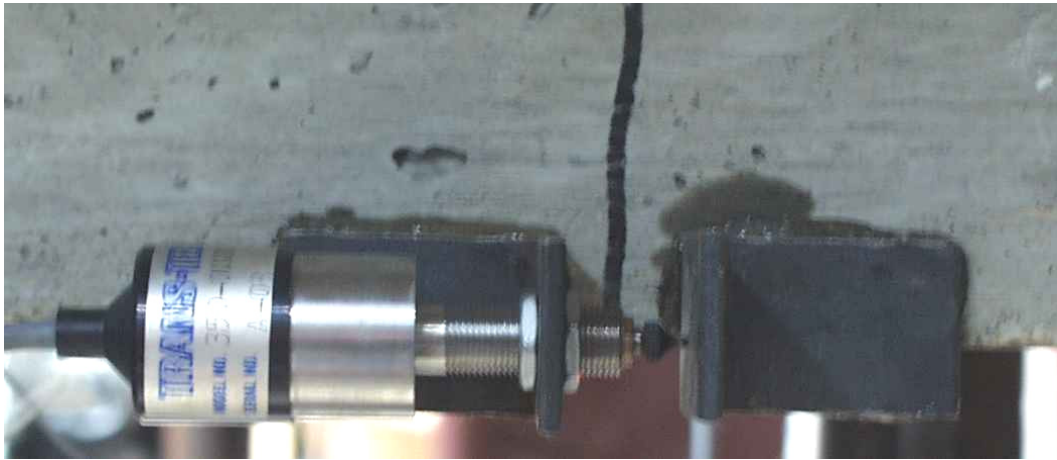
Figure 3-5 LVDT Across Crack (Crack Displacement Gage)
