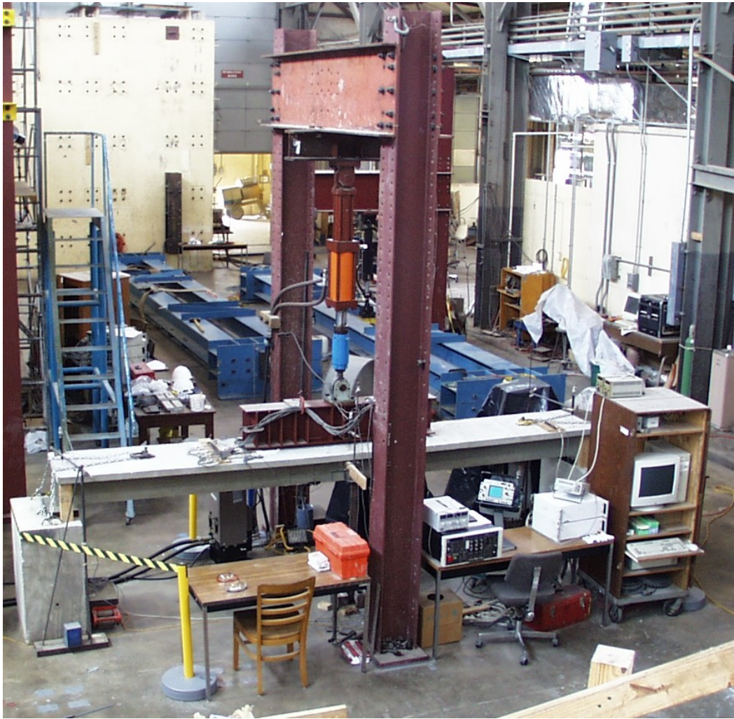
Figure 3-2 Beam Test Setup
