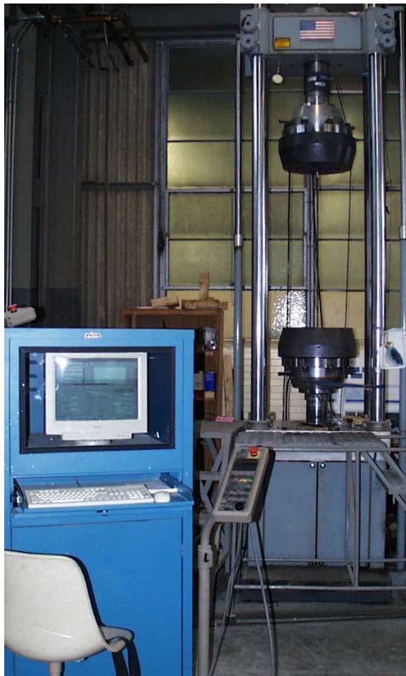
Figure 2-2 MTS Machine and Control Station
