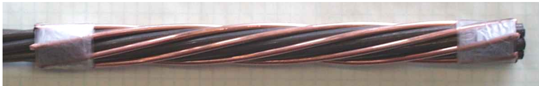
Figure B-2 Copper Wire Wrap, Ready for Installation
